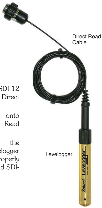
Figure 3-1 SDI-12 Interface Cable Installation
