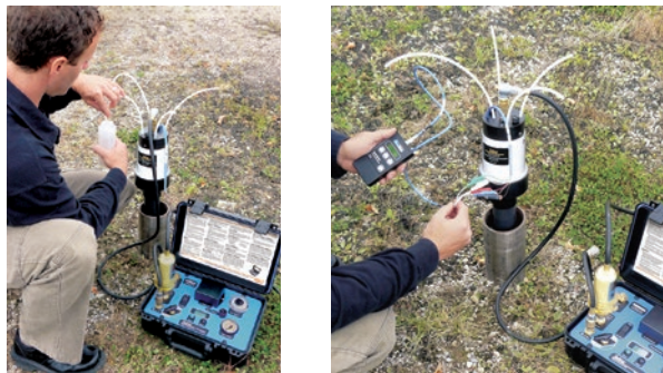
Figure 7-1 Testing Pumps and Transducers
