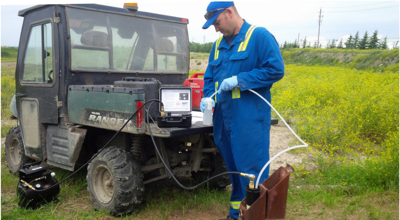
Groundwater Sampling with a Dedicated Bladder Pump using Portable, Rugged, Easy-to-use, Compressor and Controller
