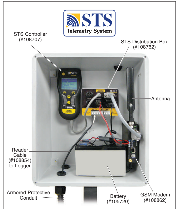
Remote Station Setup using GSM (Part#108846)
