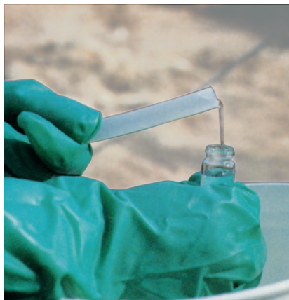
Low flow methods allow the collection of high quality, representative groundwater samples in 40 ml glass vials for VOC analysis.
