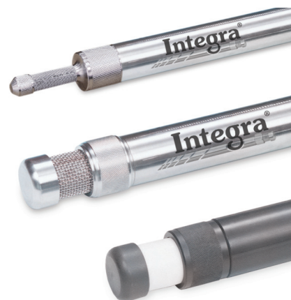
Solinst Integra Bladder Pumps are ideal for low flow sampling. Pumps are either Stainless Steel or PVC, and are 1.66" (42 mm) or 1" (25 mm) in diameter. Bladders are available in Teflon® or LDPE.
