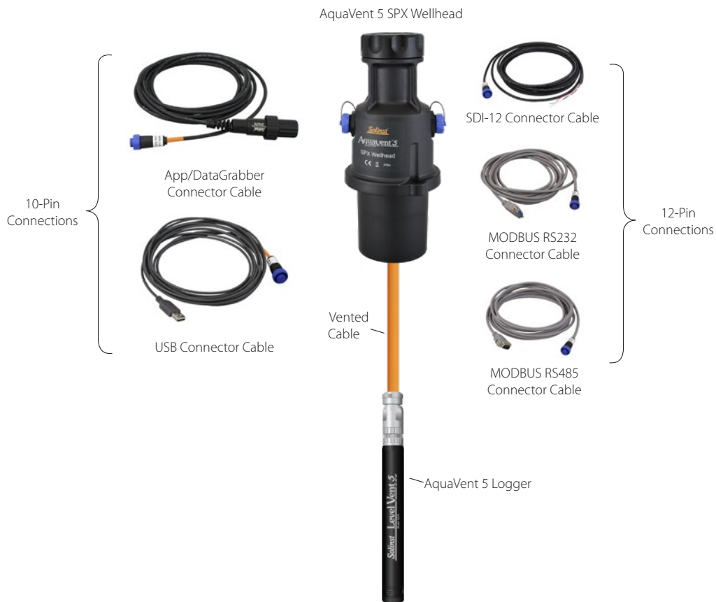
Figure 1-8 Complete AquaVent 5 System
