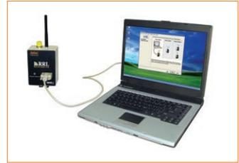
RRL Station connected to PC using RS232 cable
