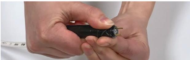
6. Use your fingers to install the new o-rings in the grooves. You can lubricate them with a bit of water if required.
