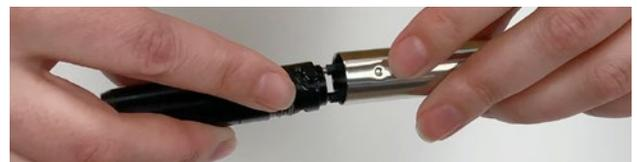
11. Line up the indents in the probe with the grooves in the tape seal plug. Push the probe past the o-rings, then twist the probe clockwise until the probe seats on the tape seal plug.
