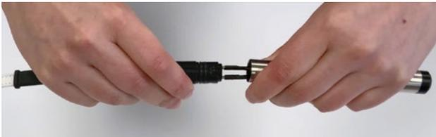
4. Remove the two connectors from the brass tubes.
