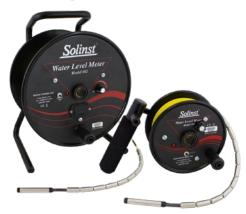
The Solinst Model 102 Water Level Meter has a new narrow cable featuring a heavy-duty polyurethane jacket. The upgraded cable is extremely durable, with extra abrasionresistance and flexibility. The yellow cable is distinctly laser-marked, offering more visibility in the field.
