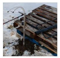
Steven Chapman, Senior Research Engineer/Hydrogeologist with the G360 Team, oversaw the installation of the Multilevel Piezometers. He noted that the "installations went smoothly". The Drive-Points consist of 3 sampling ports each and are installed to depths of ~2.2 to 2.5 meters.
