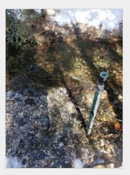
Two Leveloggers are deployed to measure the water levels on the stream. Three Leveloggers measure water levels in mine strip pits that were believed to be tied to the mine pool. Four Leveloggers are installed in boreholes drilled into the mine pool. The last Levelogger measures water levels at the Mocanaqua collapsed mine tunnel discharge.
