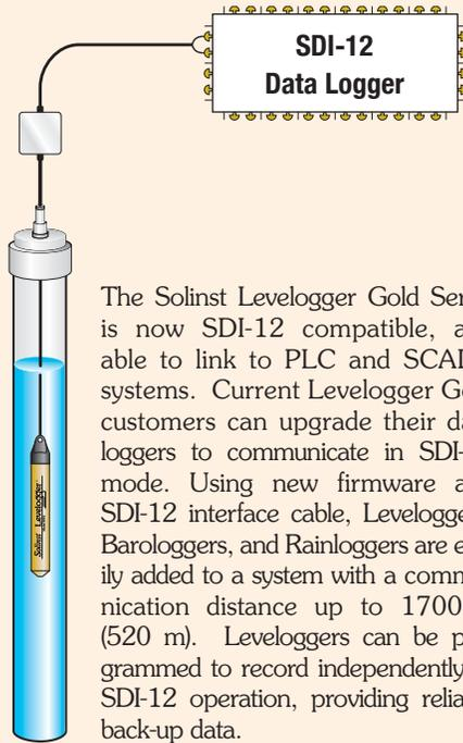
The Solinst Levellogger Gold Series is now SDI-12 compatible, and able to link to PLC and SCADA systems. Current Levellogger Gold customers can upgrade their data loggers to communicate in SDI-12 mode. Using new firmware and SDI-12 interface cable, Levelloggers, Barologgers, and Rainloggers are easily added to a system with a communication distance up to 1700 ft (520 m). Levelloggers can be programmed to record independently of SDI-12 operation, providing reliable back-up data.
