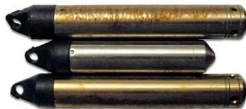
Although the data collected during the incident showed that re-calibration was definitely needed, the Barologgers continued to record in the heat of the grassfire, without much visible damage. Solinst does not recommend you subject your data loggers to such conditions, but it is nice to know these ones did *take the heat!*
