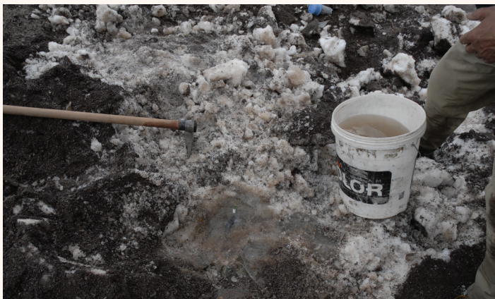
Barologger Edge still functioning after being buried in ice for over 100 days.
