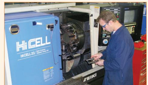
Our production area features three CNC machines (Computer Numerical Control). They allow precision machining of stainless steel, PVC, Teflon®, Delrin® and other materials, which are used to produce many of the components for our products, including Levellogger housings, water level meter probes, pumps, multilevel system components, and drive-points.
