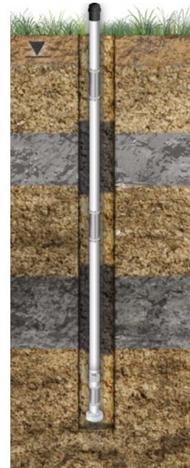
Typical 3 or 7-Channel CMT Installation using Layers of Bentonite and Sand Backfilled from Surface
