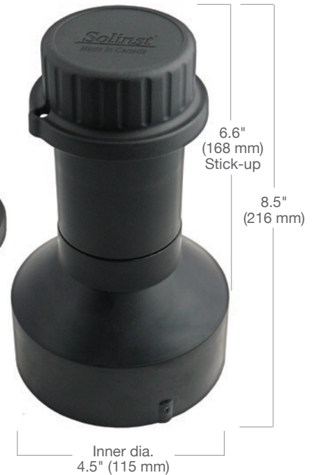
Standard 2" Locking Well Cap with 4" Well Adaptor (Fits Nominal 4" PVC Pipe)
