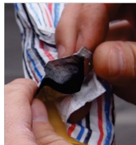
FACT Construction, with the FACT stitched between the NAPL Flute cover (striped) and a diffusion barrier (silver).
