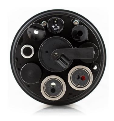
The Manta+F35 includes the same standard sensors as the +35, with the option to add up to three fluorometers. The +F35 features an antifouling copper-infused "nose cone" covering the sensor bodies. A central wiper system keeps the exposed sensor surfaces clean during continuous deployments. These features mean better data and less overall cleaning is required. PAR,  $\mathrm{CO}_2$ , TDG, and ISE sensors are unavailable on the +F35.
