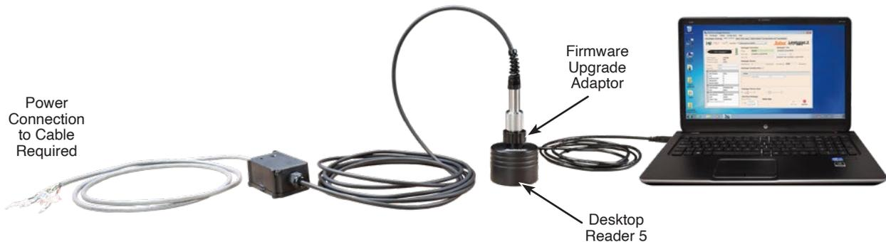
Figure 6-1 Firmware Upgrade Setup
