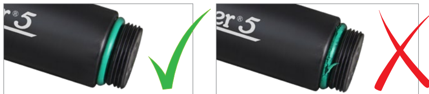
Figure 10-25 Levellogger O-ring Damage
