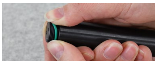
Figure 10-26 Replacing Levellogger O-rings
