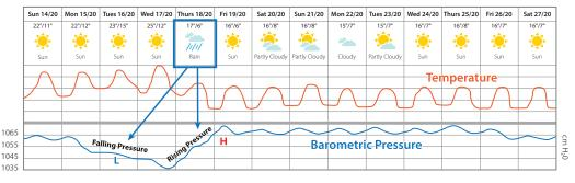
An Example of How a Storm Event Can Affect Barometric Pressure
