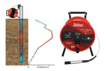
The probe is attached to high quality flat tape for depth readings, which is indicated by a light and buzzer. The tape is accurately laser-marked each millimeter or  $1/100~\rm ft$ , in lengths up to  $300~\rm m$  or  $1000~\rm ft$ . The probe and tape are mounted on a sturdy reel making operation easy. Conductivity and temperature measurements are displayed on an LCD display.
