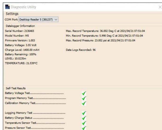
You may be able to diagnose what has caused your battery to drain, by using the Levelogger Software Diagnostic Utility. The Utility will display the temperatures your Levelogger has been exposed to, an estimate of the number of logs that were taken, as well as the battery voltage and charge levels.
