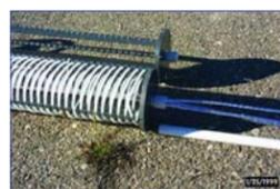
**Figure 3.** Photo of diffusive oxygen emitter
