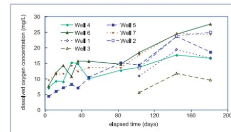
**Figure 4.** Dissolved oxygen concentrations in the emitter wells during the experiment. Only emitters 4-7 were pressurized initially; all emitters were operated. Poor performance of emitter well 3 was attributed to a pinch in the gas supply tubing to that well, which compromised the imposed diffusive gradient.
