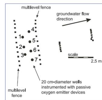
**Figure 2.** Treatment well array and ML fence configuration
