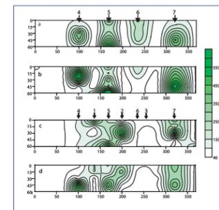
**Figure 5.** SF6 concentrations in the downgradient ML fence for snapshots 2-5. Problem associated with gas supply noted in Figure 4 is evident here in snapshot 4 and 5.
