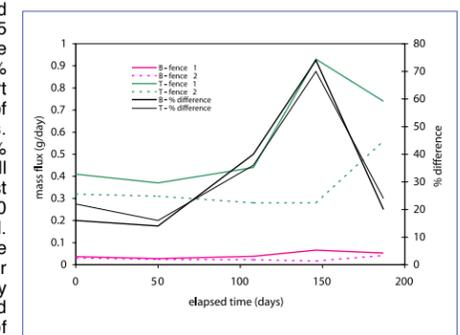
**Figure 8.** Mass flux in fences 1 and 2 for each of the five snapshot events, and the percent difference between fence 1 and fence 2 flux - an indication of treatment performance.
