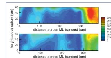
**Figure 6.** Concentration distribution of benzene in the ML fence upgradient (a) and downgradient (b) of the emitter array before the start of oxygen release.
