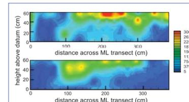
**Figure 7.** Concentration distribution of benzene in the ML fence upgradient (a) and downgradient (b) of the emitter array when all wells were releasing oxygen.
