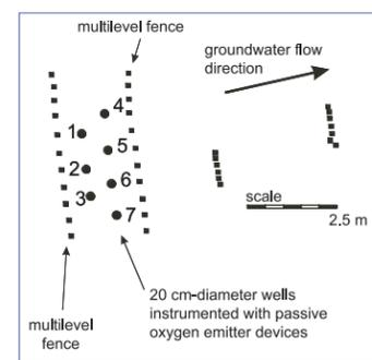
**Figure 2.** Treatment well array and ML fence configuration
