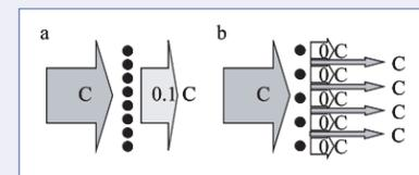
**Figure 1.** Uniform partial treatment (a) and pin stripe treatment (b), both achieving the same overall mass flux reduction. Fewer wells may be required to achieve treatment shown in (b).
