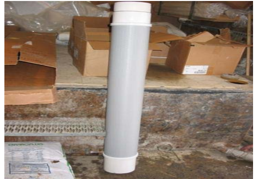
Photo 2: The 150 mm screen portion of the monitor well. Schedule 40 PVC screen was manufactured by drilling holes on the circumference of the pipe and then wrapping the solvent welding tapered PVC wire around the outside diameter of the pipe.
