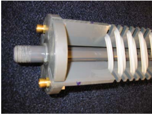
Photo 6: Close up view of the Waterloo Emitter™. Photo identifies inlet and outlet brass connectors as well as the silicon tubing.
