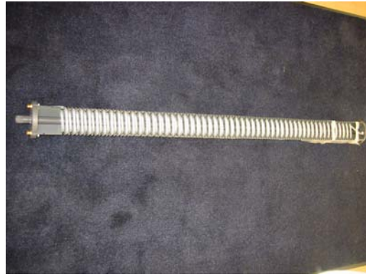
Photo 7: Full length view of a Waterloo Emitter™. Each Waterloo Emitter™ is 1.3 m in length and is comprised of a PVC frame.
