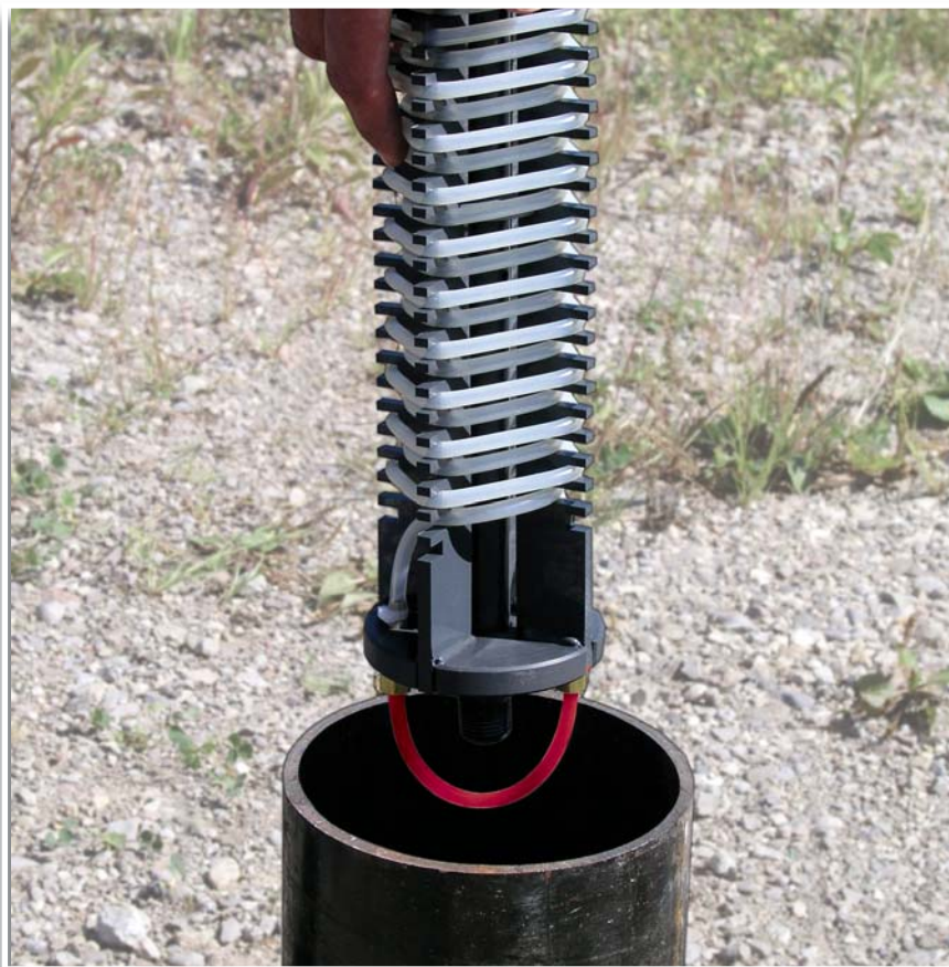
Waterloo Emitter groundwater remediation device.
