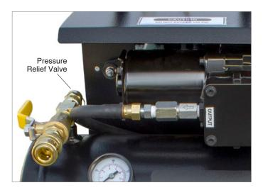
6. Test the Compressor (see separate operating instructions, if required). The 12V Compressor should turn off at 150 psi tank pressure, and on at 100 psi.
