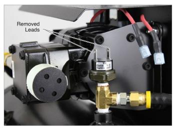
2. Use the two wrenches to unscrew and remove the old pressure switch from the brass fitting on the 12V Compressor. Use one wrench to stabilize the brass fitting, and the other to unscrew the pressure switch (see below).
