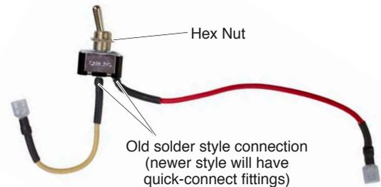
8. Connect the leads to the new on/off switch. The white lead goes to the middle terminal, and the red lead to the other.
