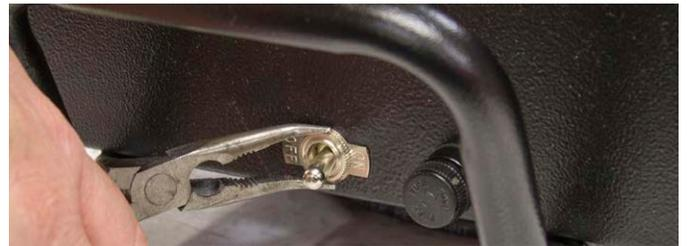
6. If your Compressor has quick-connect fittings to the switch, simply remove both leads from the old switch.
