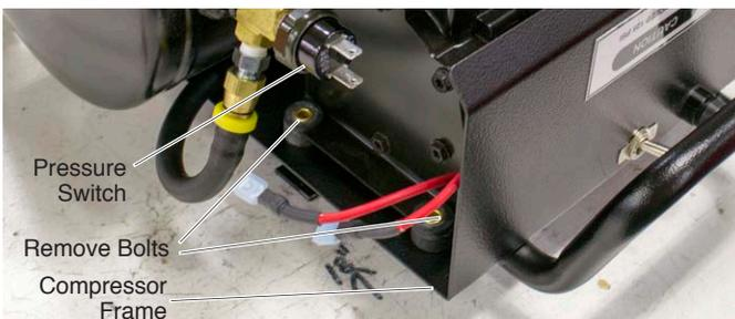
3. Remove the motor assembly from the Compressor frame. Note, the motor will still be connected to the Compressor by a black ground wire.
