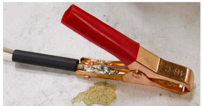
12. Slid the grips over the heat shrink and onto the handles of the new clips.
