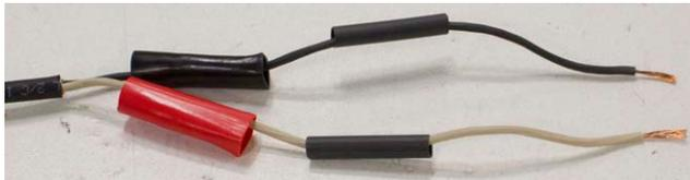
5. Slide the white wire into position in the new red clip handle. Ensure that stripped wire is showing on either side of the rounded clamp. See the photo below for proper positioning.
