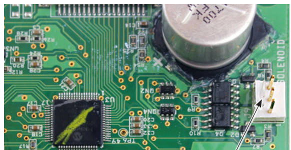
3 Pin Connector - Centre is Pin is Ground
