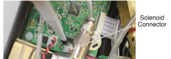
5. Carefully, pull to remove the Solenoid connector from the circuit board.
