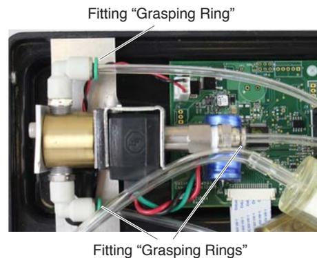
7. Use the 9/64" Allen key to remove the two screws holding the Solenoid Valve Assembly to the bracket.
