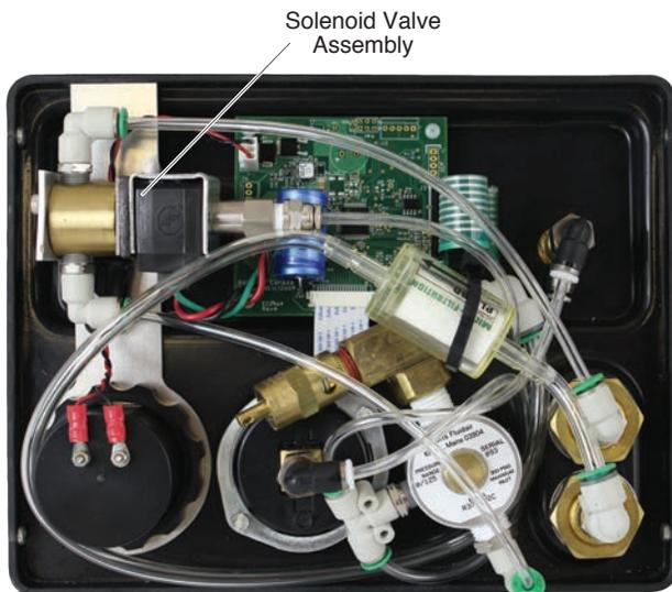
4. Use the small utility knife to break any adhesive seal that is holding the Solenoid connector to the circuit board.
