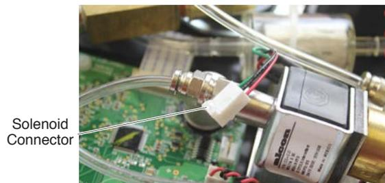
6. Remove the tubing from the three fittings on the Solenoid Valve Assembly, by pushing on the "grasping ring" on the fitting (to release tubing) and pulling the tubing out.
