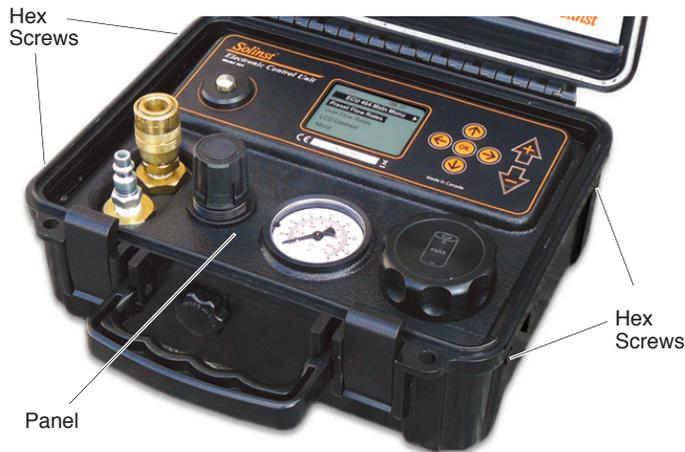
3. Remove the panel from the Control Unit and flip it over to access the Solenoid Valve Assembly.
