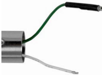
2. Use the Molex Crimp Tool (2 mm position - see photo at top) or suitable pliers to connect the crimp terminal to the wire. Tug the crimp terminal to ensure it is securely attached to the wire.
