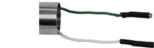
7. Slowly twist the probe up to two times. This shortens the wires and allows them to tuck easier into the probe body.
