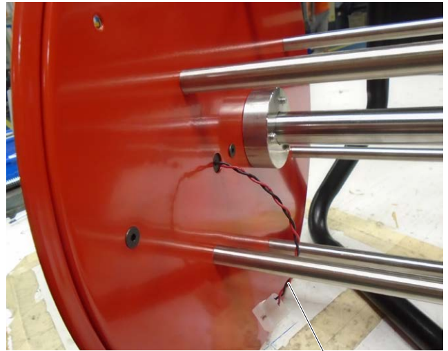
Secure wires with Molex connector to a spoke
