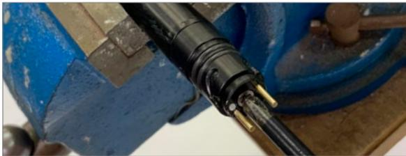
5. Use pliers to pull out the two brass tubes and the black disk from the tape seal plug.
