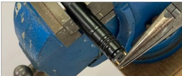
6. If this is a newer style tape seal plug, remove the two o-rings from the openings.
