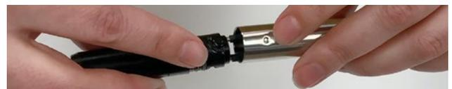
15. Line up the indents in the probe with the grooves in the tape seal plug. Push the probe past the o-ring, then twist the probe clockwise until the probe seats on the tape seal plug.
