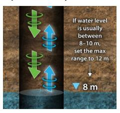
In general, knowing the approximate water level before measuring allows you to set a minimum depth to start detecting, and a maximum depth to listen for the returning pulse. For example, if depth to water is usually between  $8-9~\mathrm{m}$ , set your minimum to  $7~\mathrm{m}$  and your maximum to  $10~\mathrm{m}$  for higher accuracy.
