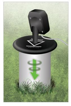
The seal around the probe does not have to be airtight, but the signal works better when the sound waves cannot escape and it also helps prevent external noise, such as wind, from interfering with the sound wave.
