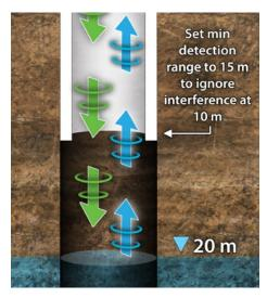
**Note:** a drop tube should be used if there are more significant disturbances in the well, such as a large step-down in well casing diameter or perforated casing sections.
