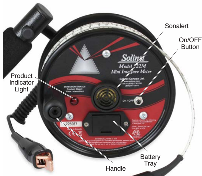
122M P8 (CSA) Mini Interface Meter indicating the location of components
