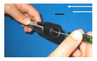
Insert the screwdriver blade through the hole in the locking nut to reach the adjustment screw.
