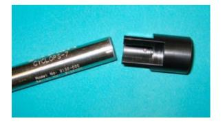
Align the index mark and indexing ball when installing the chlorophyll sensor in the Solid Secondary Standard.
